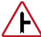
Approach to intersection side road
