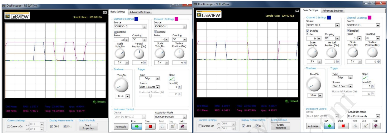
Figure 1: The PCM Encoder module's PCM Data output at 1V and 1.5V respectively.
