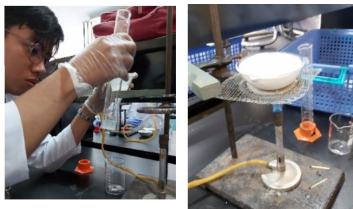
Fig. 1. (a) water filtration; (b) evaporation of the water sample.
