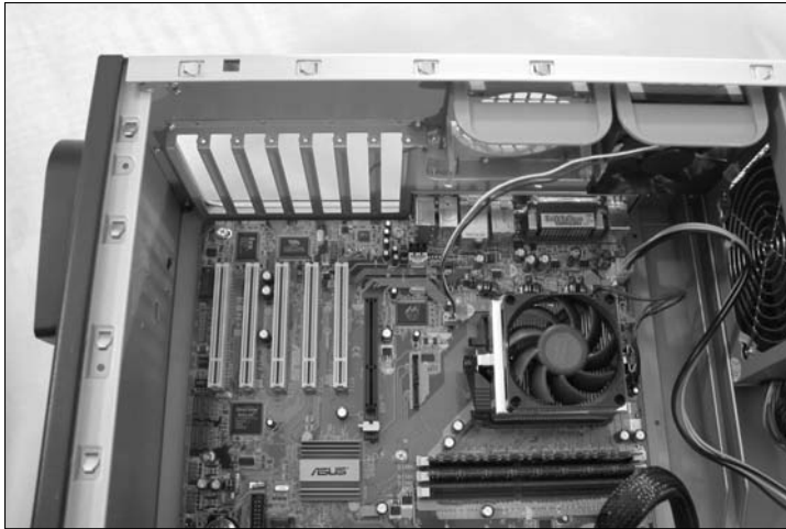
Figure 4-1: Your goal: The motherboard, CPU, and RAM all installed.
