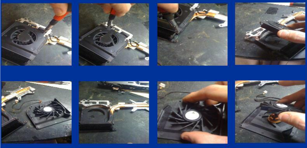
More Pictures of Fan/Heat-Sink Cleaning
